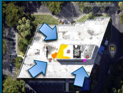
Aerial Infrared Identifies Hidden Moisture Damage
