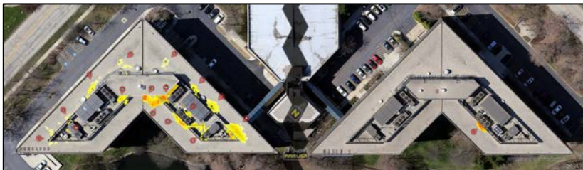
Blended Image – Pinpoints thermal anomalies in need of further investigation
