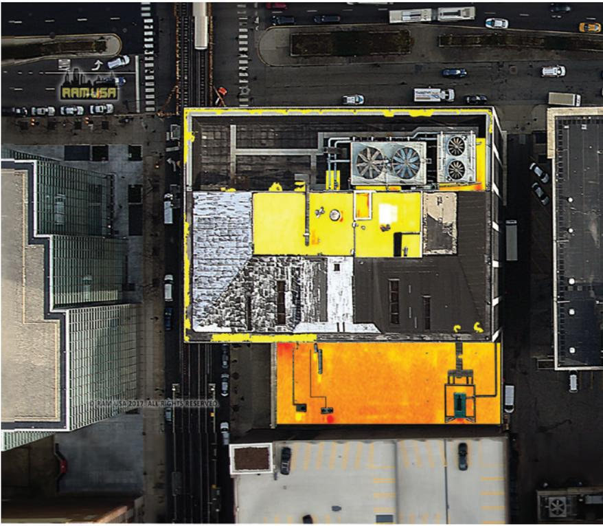
**LOOKING INSIDE** Aerial infrared scans have proven to be an effective way to locate hidden moisture within a roof system.
