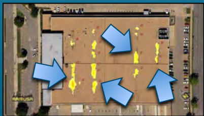
Aerial Infrared Identifies Hidden Moisture Damage
